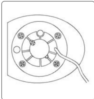
3. Attach the front and rear bases to the underside of the fan using the four cross recess screws. Make sure that the front and rear bases are securely fixed to the fan.
